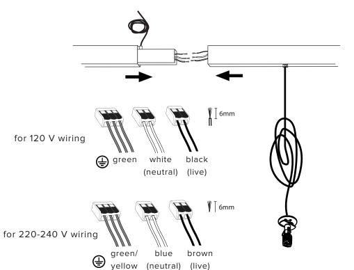
Carefully place wires and Wagos in between connecting plates of the bars before sliding the bars
