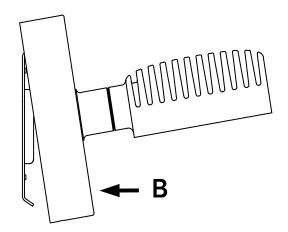
Push the bottom part of fixture against the wall.
