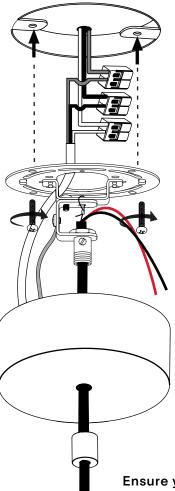
Connect luminaire's red and black wires to driver output wires (DC) within the canopy.
