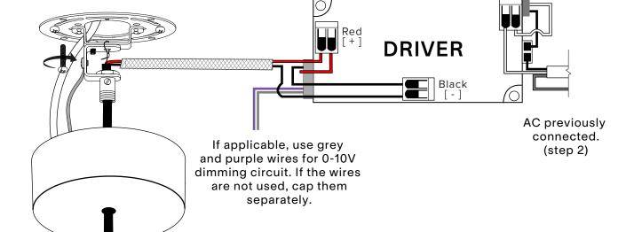
Ensure your electrical box can hold a weight of 35 lb/ 16kg and that no wires are pinched during these steps.
