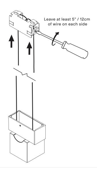
through anchor cover, make sure the set screw hole is facing the closed side of the bracket.
