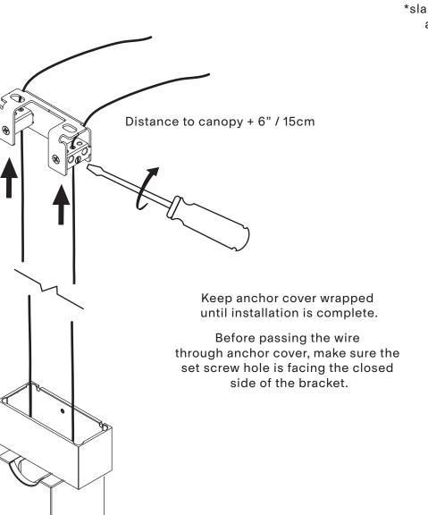
\*slab follows the same steps as non-electrical side Leave at least 5" / 12cm of wire on each side When desired height and level are achieved, tighten the strain reliefs. ◙▥∅
