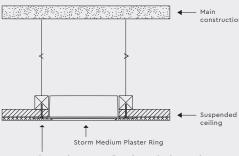
Make sure the Storm Medium Plaster Ring is securely fasten to the reinforcement.
