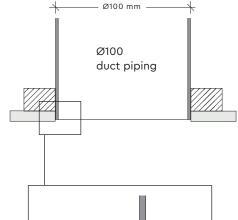
Make sure the ventilation ducts pipe's outer diameter fits the hole in the ceiling.
