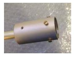
Adjust the adjustable screws to the glass ball opening. There has to be a minimum of 1 mm distance between the metal and the glass
