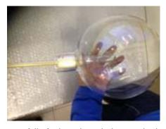
Carefully fix loosely with the supplied knurled-head screw by hand. Do not use a screw driver. Do not screw too tight, ensure there is at least 1 mm tolerance between the glass and the screw
